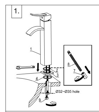
1.Make a hole of Ø32~Ø35 on the installation plate, screw off the hexangular nut(7) from the long rod (8), then screw the inlet pipe(9) and the long rod (8) onto the main body(1).
