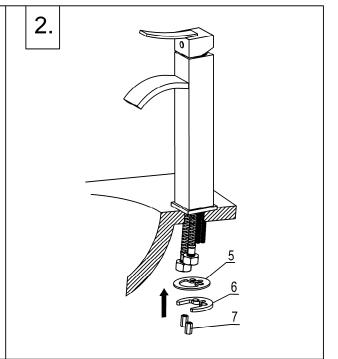
2. Fixing the faucet from downside of the installation plate, with the 2-hole washer(5), 2-hole gasket (6) and the hexangular nut(7).
